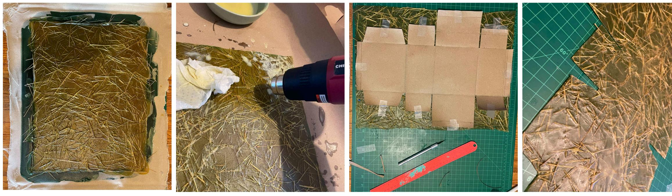
A sheet of the fiber composite is made. Beeswax is added to the inside for additional protection, waterproofing, and rigidity.
