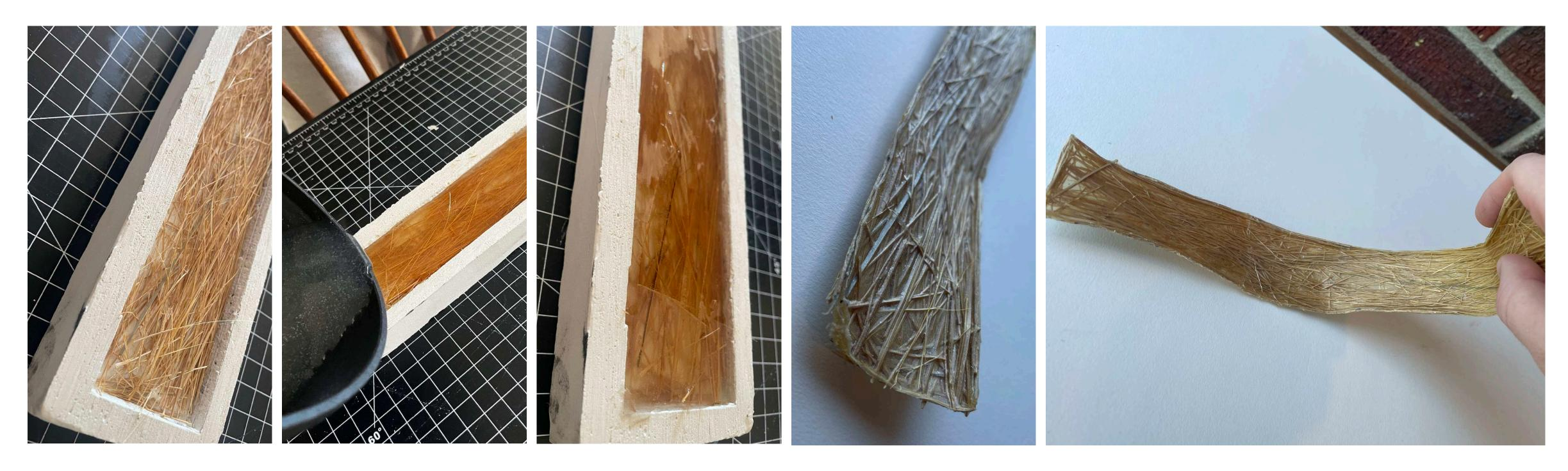
The material is flexible and very strong. The agar shrinks around the bamboo fibers while they minimize the overall shrinking of the material. It can be bent without snapping or tearing.
