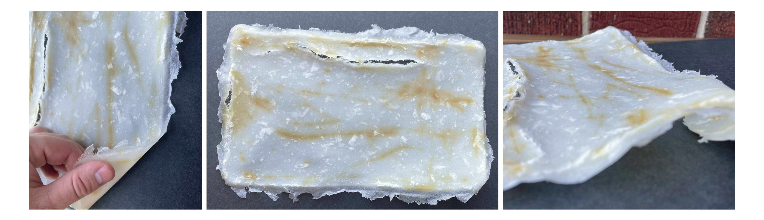
This recipe was overall very successful. The leather is fairly strong and pliable with a little elasticity. The material does take a while to dry, almost a week. There was a tear in the material while drying due to the shrinking while the water evaporates out.
