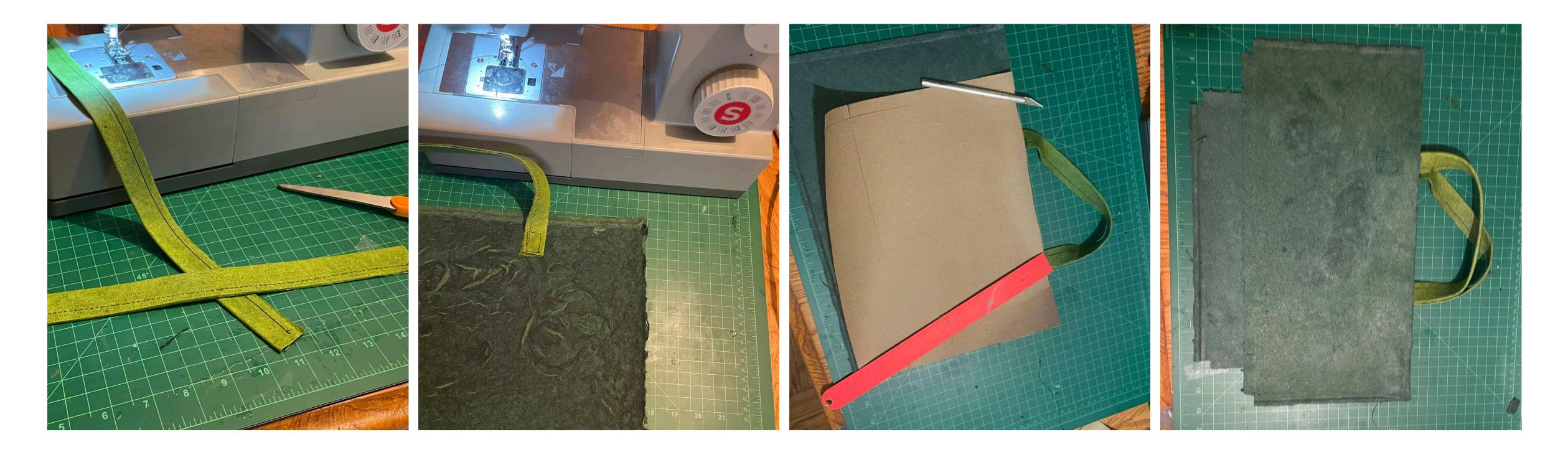
I tested sewing the cellulose leather and other methods of construction. Unfortunately, the more I worked with the material the weaker it became. It is fragile and prone to tearing. An increase in agar concentration could potentially strengthen the material and solve this issue.
