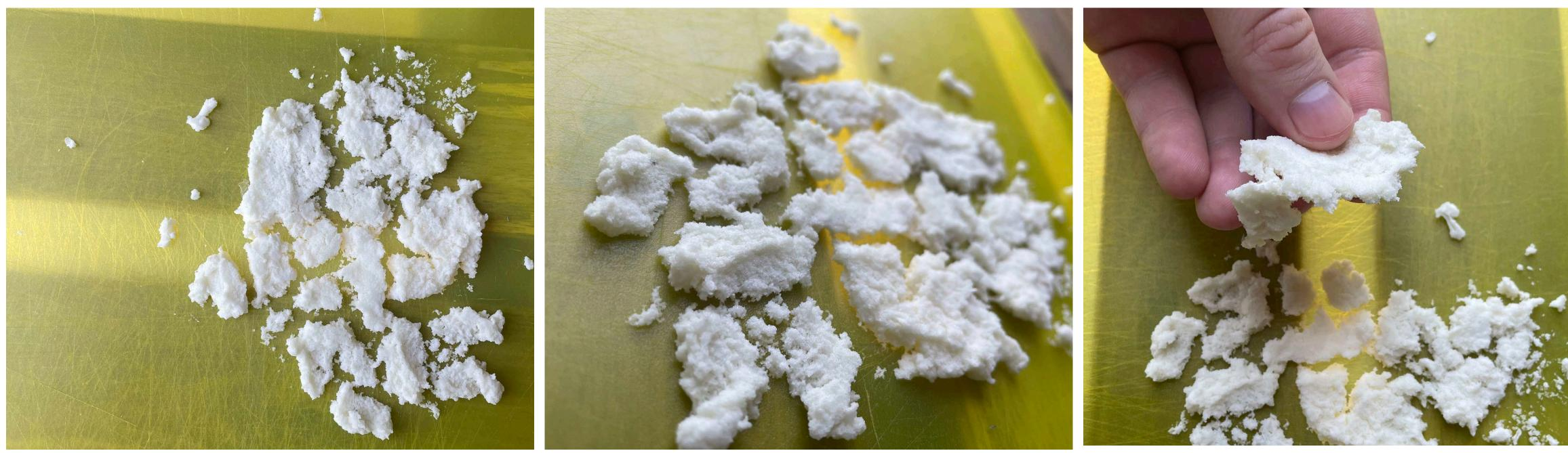
This material was not very successful. It takes a while to dry, and does not offer any strength or flexibility. The material is very brittle and fragile, crumbling during the drying process. It can also not be handled without breaking.
