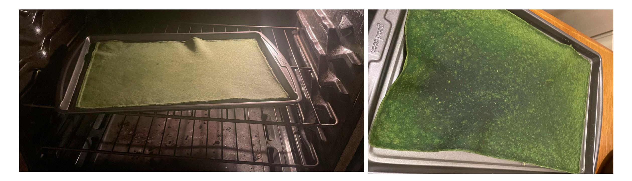
The final cellulose leather recipe replaces cornstarch with agar, but keeps the pulp as the fiber.
