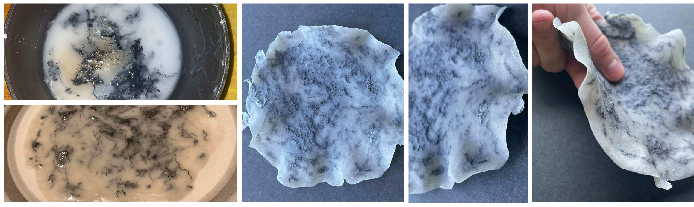
This material was successful. It has a similar soft feel to the previous cellulose leather, but is more elastic and pliable. It dries much quicker thanks to the addition of agar. The cotton fibers distribute stress more evenly along the material and there were no cracking problems. It does have similar curling to the previous agar material.
