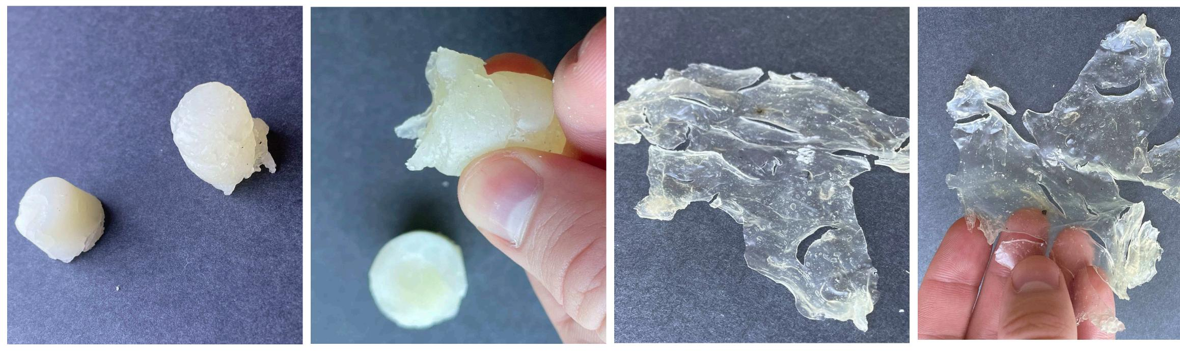
This material was not very successful. It is soft and brittle, crumbling easily both during the drying process and while handling when dry. This problem is evident both when molded and dried flat.
