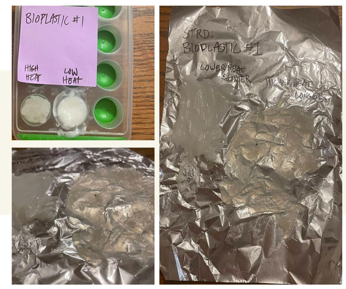
2 tests were done, one at higher heat and becoming thicker and the other at lower heat and not thickening as much. Both tests were poured in small mold and spread flat onto foil
