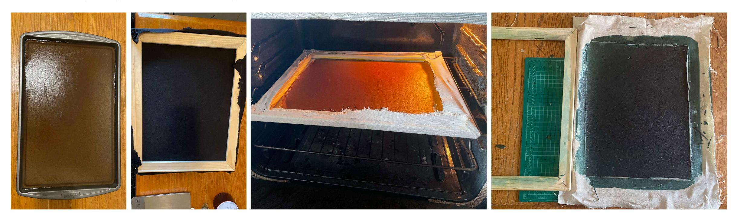
I first tested a sheet pan with another weighted sheet pan on top, dehydrating in the oven. The stacked sheet pan did not let enough water to escape but the material would curl without it.
