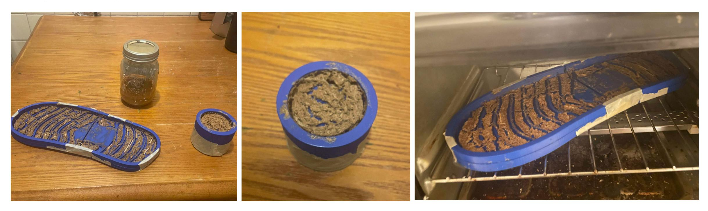
To reduce drying time and solve shrinking, I tested pouring small layers of the bamboo and agar composite in 3d-printed molds and then dehydrating them. When a layer is done drying, I add another to unite the shrunk pieces.
