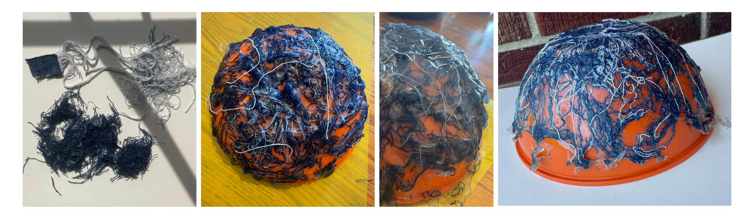
Using scrap denim, I seperated the fibers. There are much thicker and sturdier than the cotton T-shirt fibers I used. I tested a composite with the agar plastic poured over the outside of a round form to see how it shirnks and curls around it.
