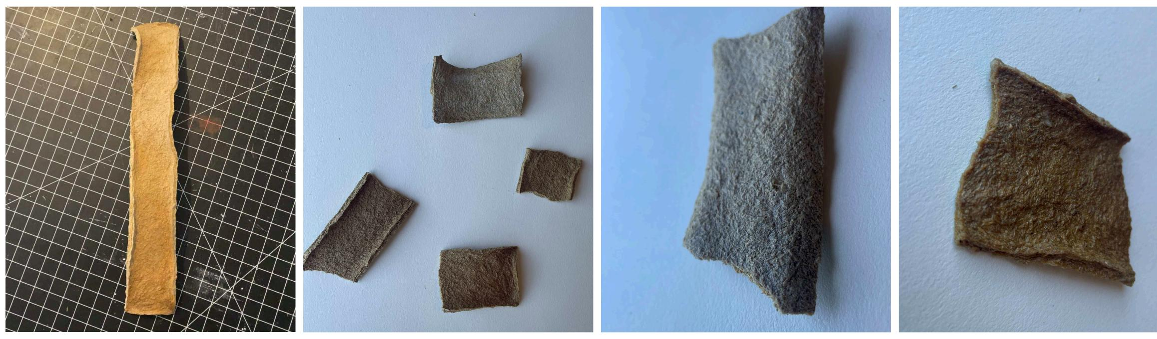
When dried, this material is very rigid and hard. This is a successful breakthrough in finding a material that has some of the rigid properties of plastic. It is somewhat easy to snap when thin and has some curling and shrinking issues.
