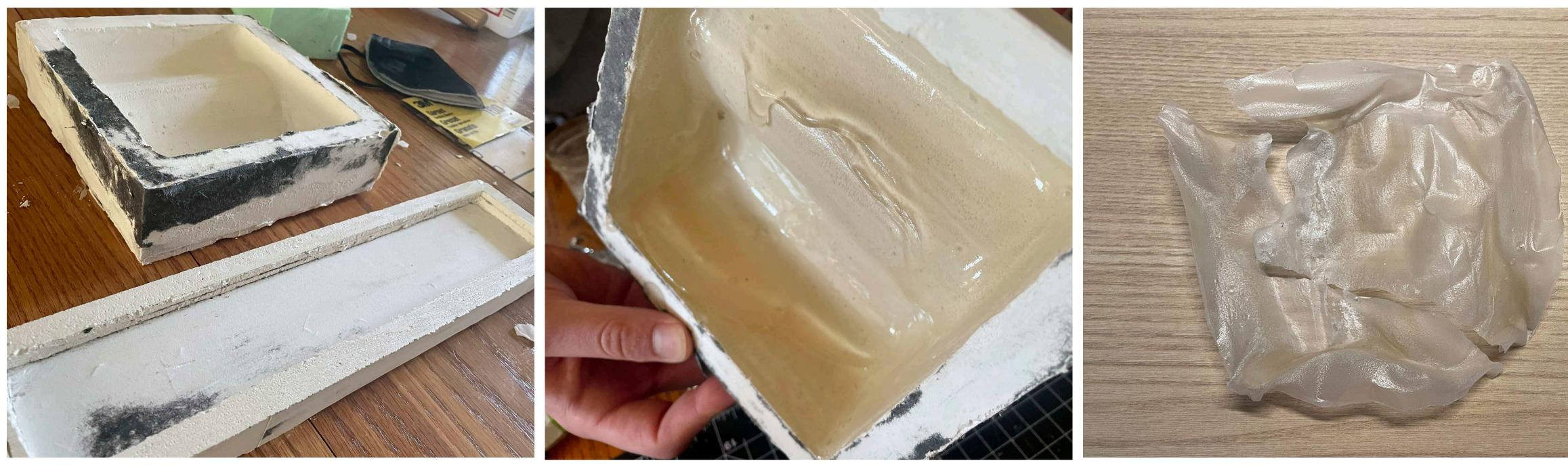
The first mold test I did was using my standard agar recipe as a thin film over a curved mold to see how it holds a shape. The material shrunk but held a form and was more sturdy than plastic wrap.
