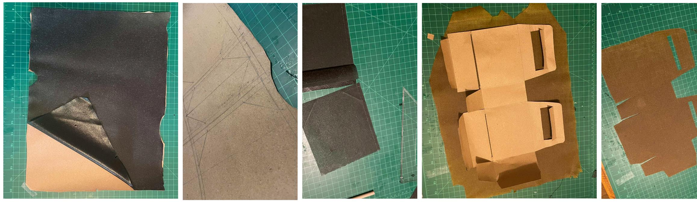
First, paper prototypes and patterns are made within the constraints of the plastic sheets. The bioplastic is then cut into the pattern and made into packaging and prototypes.
