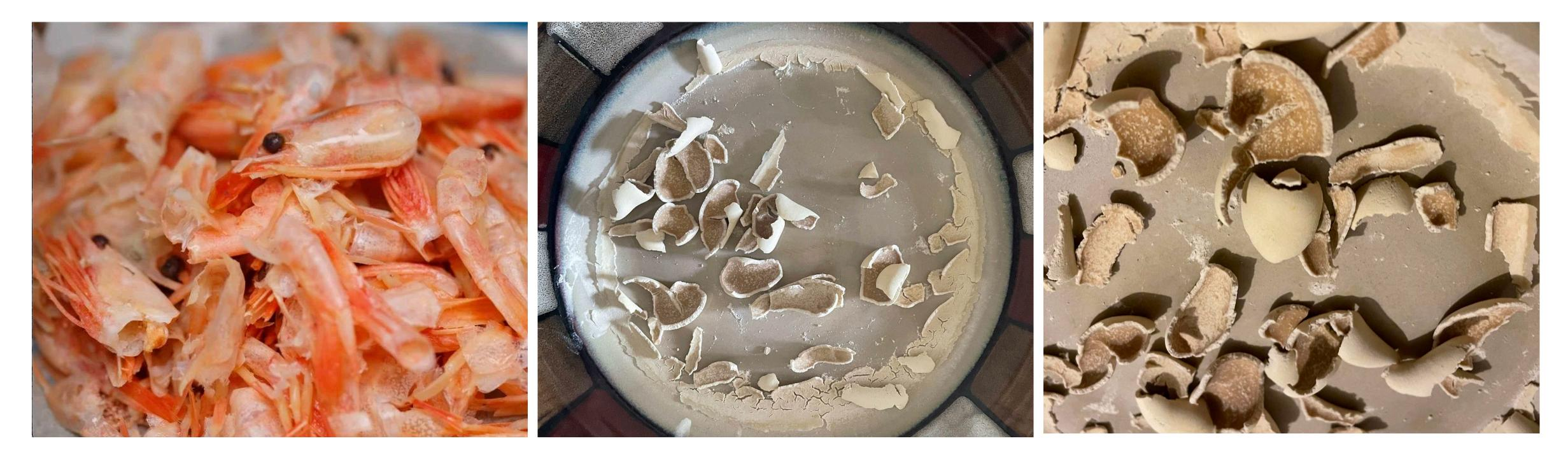
I combined chitosan powder with water and glycerin and heated the mixture. It was unsuccessful. The material is powdery, dry, and crumbly. It shrunk and broke apart during the drying process.
