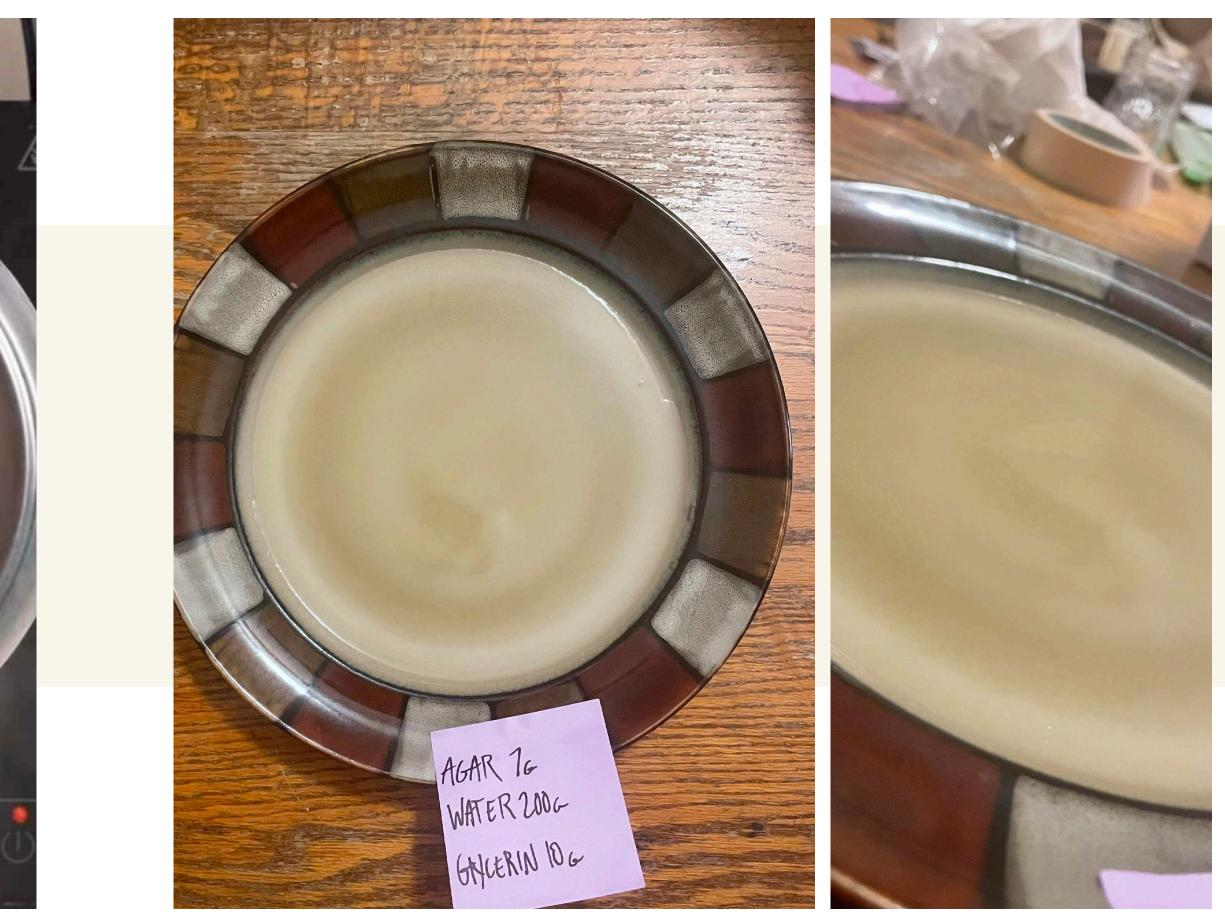
Mixture poured into shallow plate as mold. The material is almost completely clear and quickly firms up
